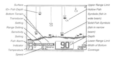
The Wide Vision allows you a number of ways to display sonar information. Some features are used in conjunction with special accessories such as the Boat Speed and Water Temperature gauge, or "Wide Side" side looking transducer.
